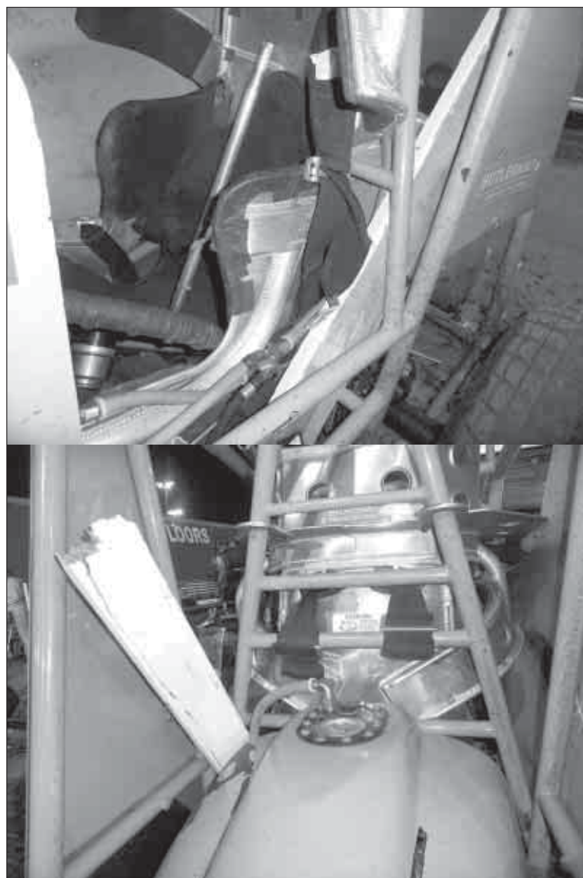
These photos show the 2x4 that entered the cockpit of Austin Johnson's Sprint Car at Knoxville Raceway
